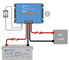
System with DC-DC converter, providing galvanic isolation between the battery and the DC load or circuit.
